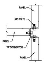
3-Way Panel Connection with U-Channel (3/8" Diameter Bolts Shown)
