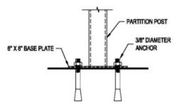
Partition Post Base Anchoring Detail
