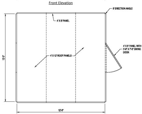
Kelly Klosure Expanded Metal panels can be installed with partition posts to create an enclosure or wall system with no roof or upper supports.
